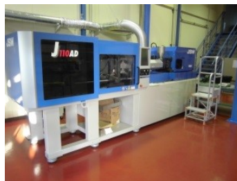
Injection molding machine (for preparing test specimens)
